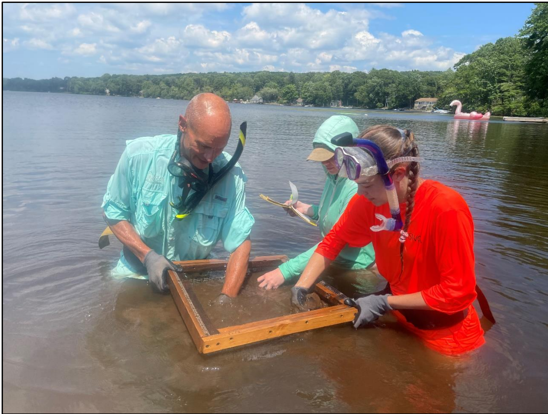
Photo A-1. Sifting a quarter-meter sample at a water depth of three feet.
