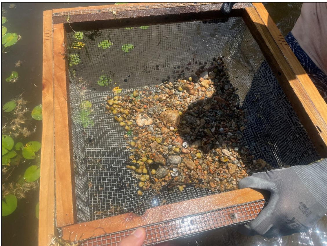
Photo A-2. Quarter-meter quadrat sampler (2.69 square feet) with \frac{1}{4} inch mesh.
