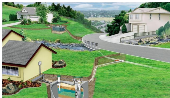
Typical STEP Sewer Configuration. Source: http://www.orenco.com/systems/wastewater_collection.cfm
