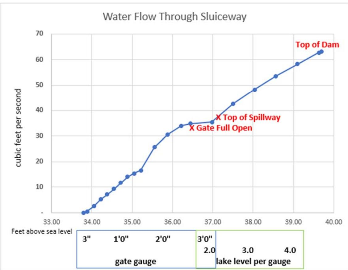
*Note: Water flow increases as the lake level rises, the higher water level increases water pressure*
