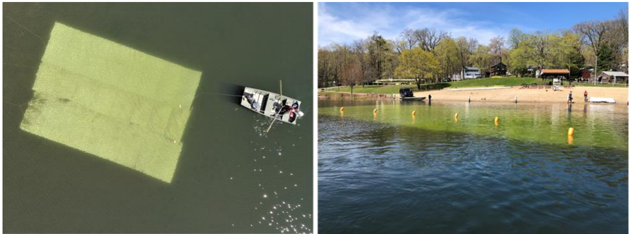
Figure 8. CAES IAPP testing of short-term benthic barriers in Lake Beseck.
